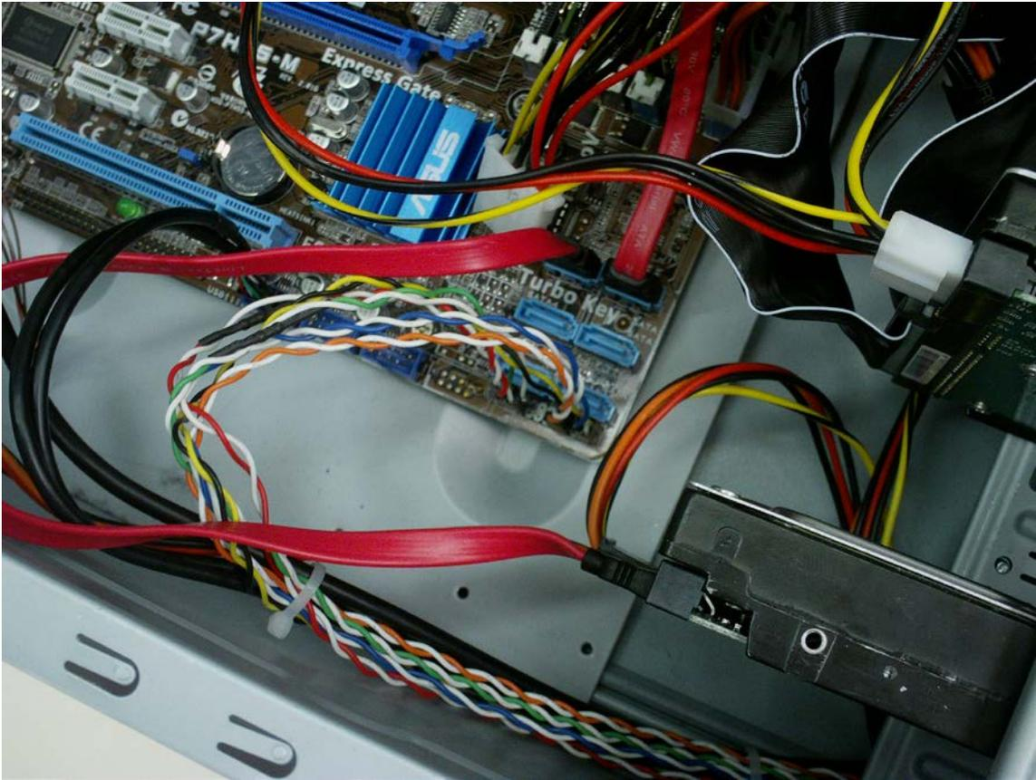
**Figure 10** - System panel LED connections
