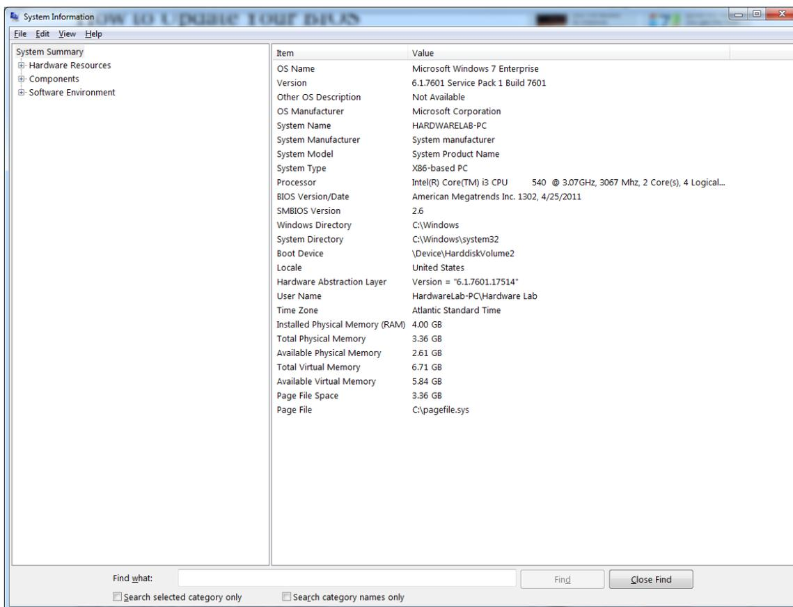
**Figure 11** – The System Information (*msinfo32.exe*) window. Make note of “BIOS Version/Date”, here appearing under the processor information.
