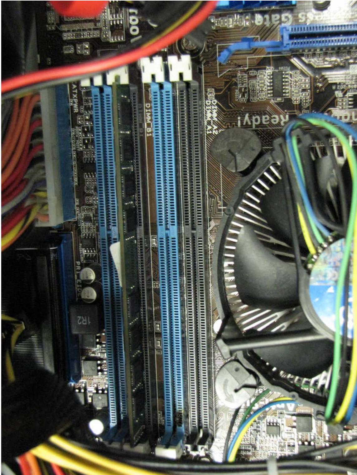
**Figure 7 - RAM slots (these slots support dual channelling)**
