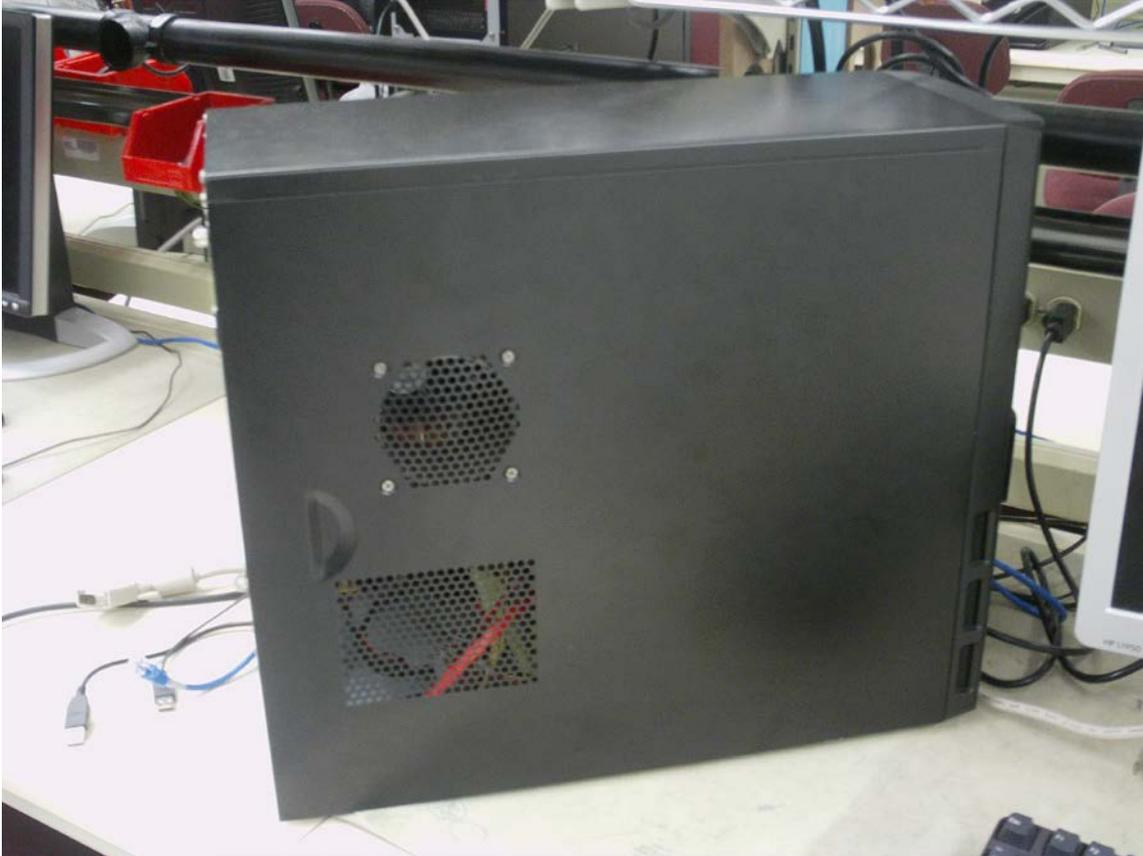
**Figure 2** - Case cover designed to slide off
