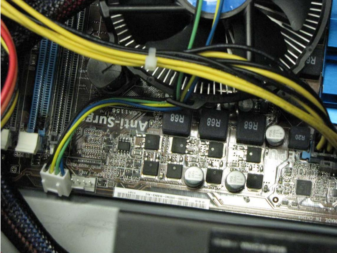
**Figure 6** - Disconnected CPU cooling fan. Ensure that its power wires are connected to the motherboard (lower left)
