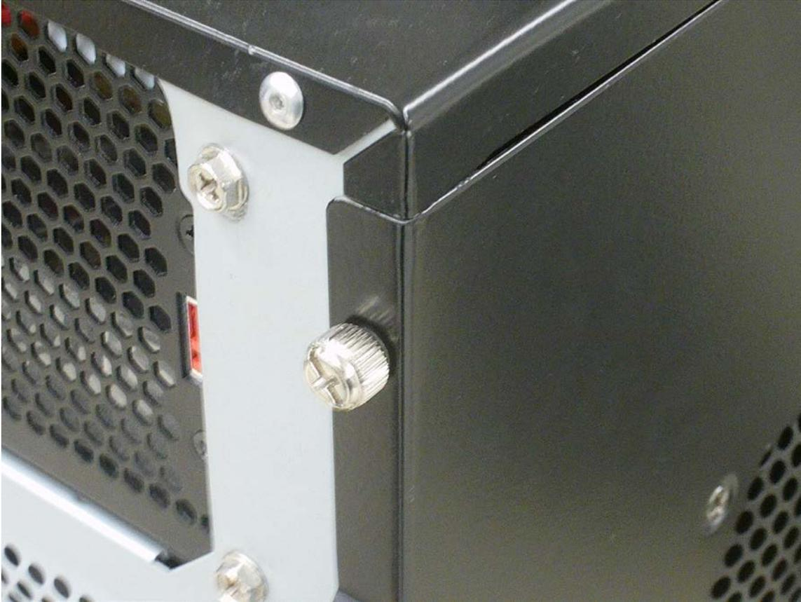
**Figure 3** - Case cover screw that can be removed with one's fingers
