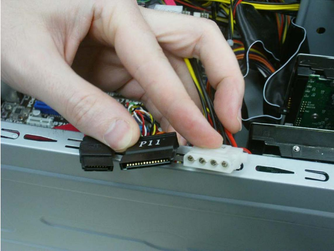
**Figure 9** - Hard drive connectors, from left to right: SATA, SATA power, Molex 8981 (choose one and only one of the latter two)
