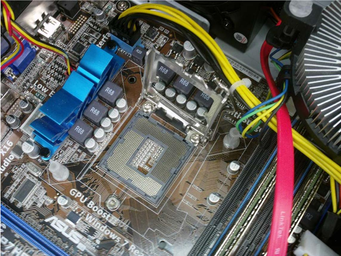
Figure 4 - Opening the CPU socket
