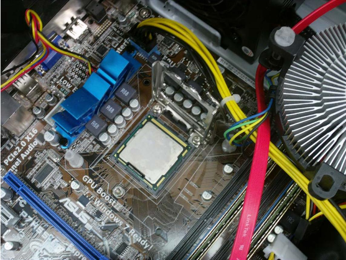
**Figure 5** - The new CPU placed in the socket; thermal paste applied
