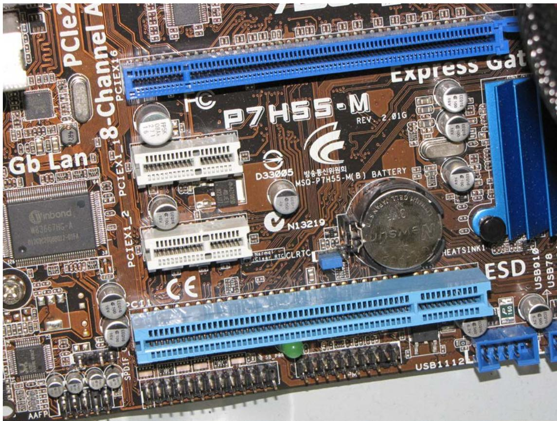
Figure 12 - The CMOS battery and the settings jumpers (to its lower left)
